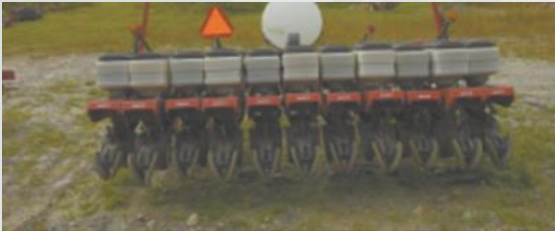
In addition to higher yields, Wallace says he uses less seed since he started planting wheat with a corn planter fitted with inter-plant row units.
